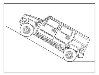
Design specifications required a minimum gradeability of 60% (31 degrees) slope, with the vehicle fully loaded, on high friction surfaces with maximum vehicle speed not to exceed 6 mph (9.7 km/h). The vehicle is expected to traverse this grade only for short durations. Never stop and idle the vehicle or park it on this grade.
